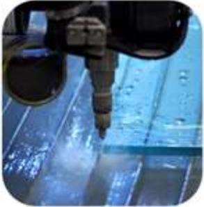
**5-axis** waterjet cutting with up to **64°** **incline** can cut almost any material up to **200mm thick**
